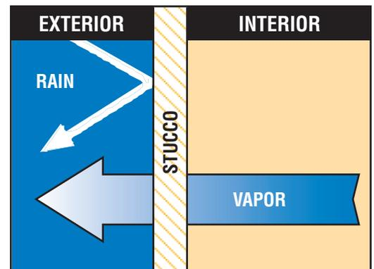
The Loxon system allows the coating to resist wind driven rain. It also allows the masonry structure to release moisture vapors without interfering with the adhesion and the performance of the coating.
